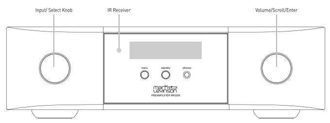
The Mark Levinson team designed the  $N^05206$  for elegant simplicity and ergonomics; therefore, the knobs perform a variety of functions depending on the operating mode. There are two modes of operation, *Listening* mode and *Setup* mode, and three modes of *Standby*, Green, Power Save, and Normal.
